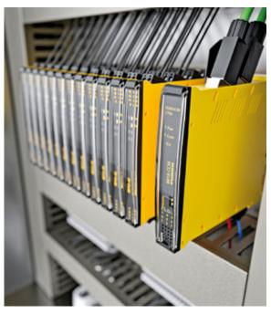
The IM18-CCM transfers measured values via Ethernet to IT networks and can even preprocess them remotely
