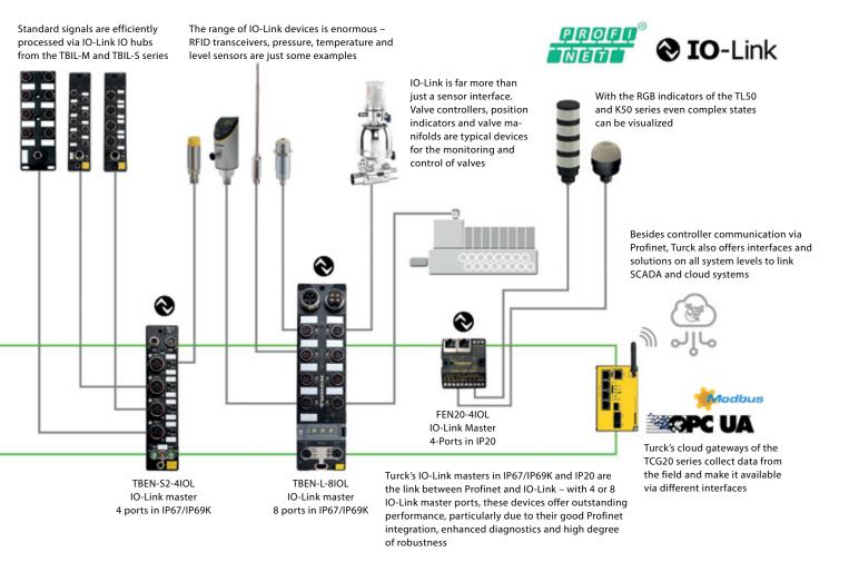
with SIDI give IO-Link devices the identity of a genuine Profinet module with their own GSDML entry. The function considerably simplifies the engineering of IO-Link devices in projects with Profinet controllers, since it allows access to all parameters and device properties from the engineering system without the need for additional software.
