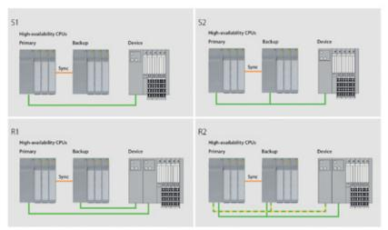
Redundancy principles: S1 is a simple connection, i.e. no redundancy; if a Profinet device communicates with the primary controller and its backup via this connection, this is classified as S2 – very high and maximum availability is offered only with R1 and R2 system redundancy, which also require dual systems on the field side
