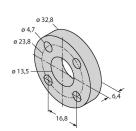
Standard spacer made of nonferrous material for separating the positioning element from the base of the hydraulic piston rod
