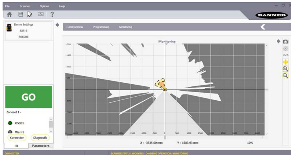
Figure 12. Monitored space as shown by the SX5soft software
