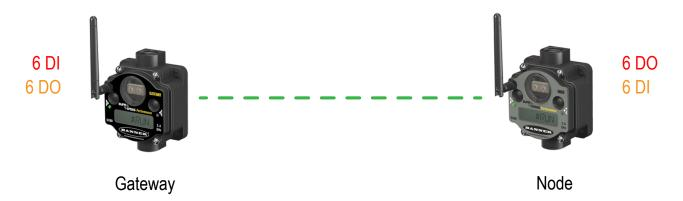
The SureCross® Performance Mapping kits create a radio frequency network with integrated I/O that can operate in most environments and eliminate the need for wiring runs. The Performance Mapping kits include one Gateway, which acts as the wireless network master device, and one Nodes. I/O mapping between the Gateway and Node are set using the Gateway's DIP switches.
