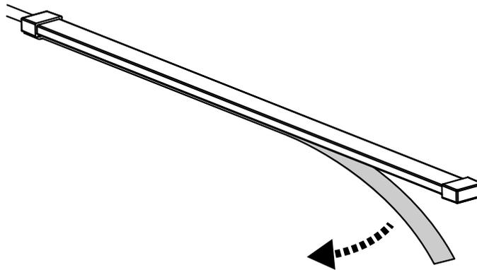
3. Align the light strip in the desired installation position, and press the light strip firmly onto the mounting surface. After installing the light strip, wait twenty-four hours for the tape to adhere completely to the mounting surface. Do not touch or move the light strip during this time period.
