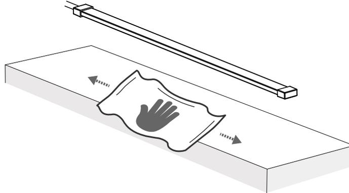
2. Remove the protective liner from the tape on the back of the light strip.
