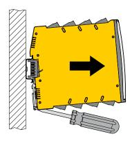
Fig. 4: Remove device
