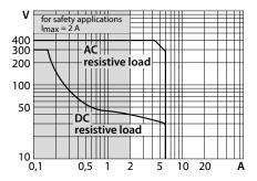
Fig. 7: Output relay load curve
