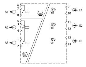
Fig. 5: Block diagram IMX12-CD01-2R-2U
