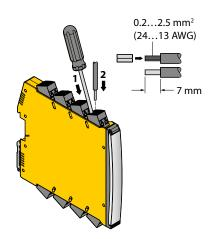
Fig. 3: Connection with spring-type terminals
