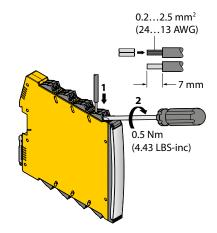
Fig. 2: Connection with screw terminals
