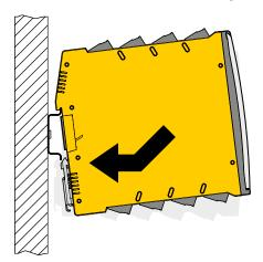
Fig. 1: Fasten the device
